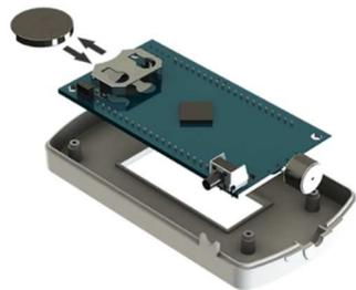
2° Carefully remove the electronics of the case and push the lithium coin out of the holder.
