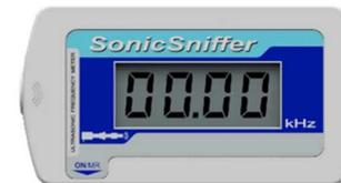
**2°) Measure:** Move it to a distance of 10 cm (4 inches) from the horn (tool, sonotrode).
