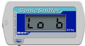
The equipment operates with a lithium coin model CR 2032 (3V). Replace the lithium coin when display shows the message "Lo b" (see image). This message means the lithium coin is depleted (voltage below 2.3 Volts).
