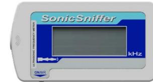
**4°) Turn it off:** Press and hold the ON/MR button to turn the equipment off. Otherwise, the auto-shutdown function will turn it off automatically after 3 minutes in idle.
