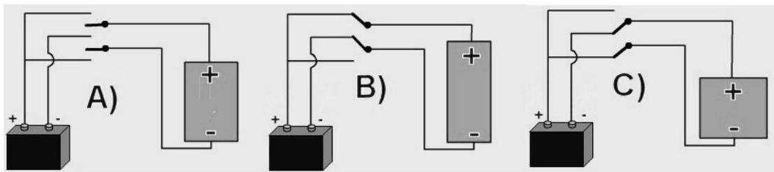
Figure 3 - Inverse piezoelectric effect in a piezoelectric ceramic rod polarized on the length: An electric field applied in accordance with the field used in the polarization causes it to stretch, and a field with reversed polarity, to contract.
