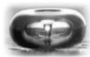
Figure 12 - Photo of the initial moment of the collapse of a cavity.
