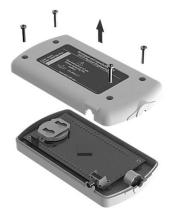
The meter operates with a lithium coin model CR 2032 (3V). Replace it when display shows the message "Lo b" (see image). It means "Low battery" (voltage below 2.3 Volts).
