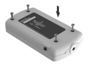
$5^{\circ}$ ) Attach the case bottom (9) and close the set. Insert and tighten the screws (6) until fix the case firmly.
