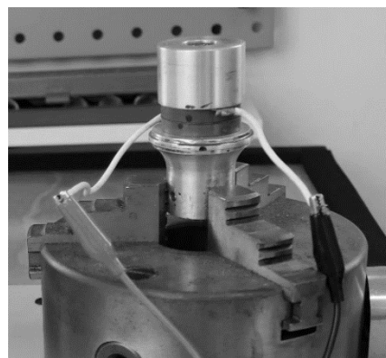
Electrical connection between PiezoClamping and the transducer.
