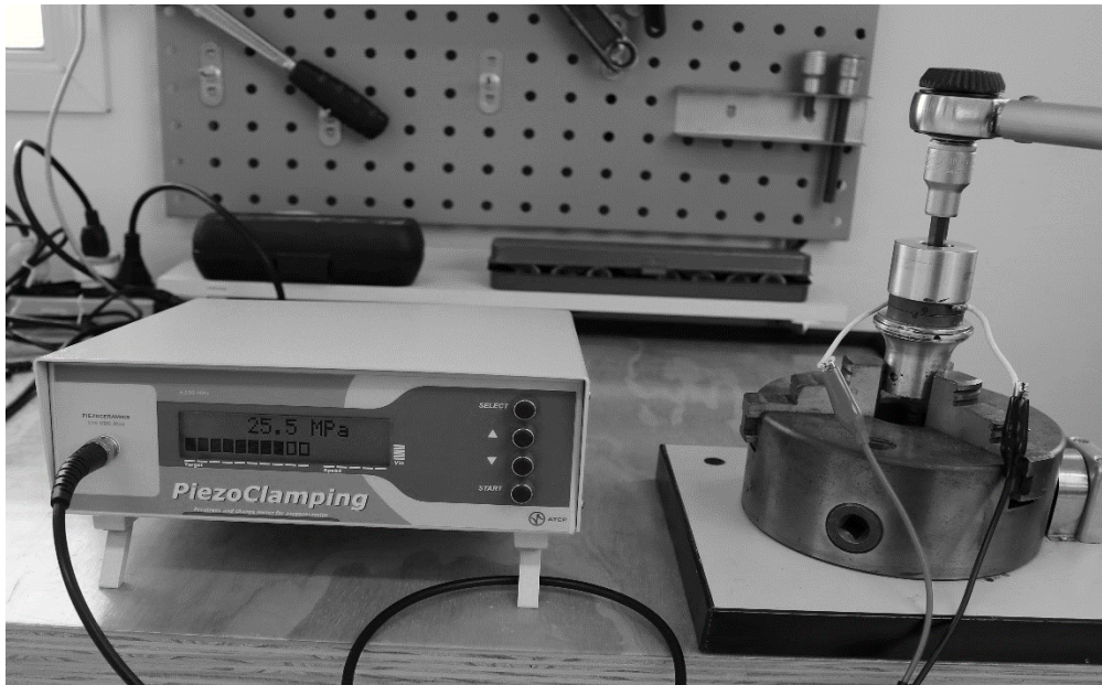
PiezoClamping connected to control the prestress of a converter.
