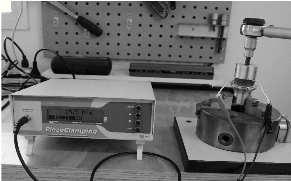
PiezoClamping connected to control the prestress of a converter.
