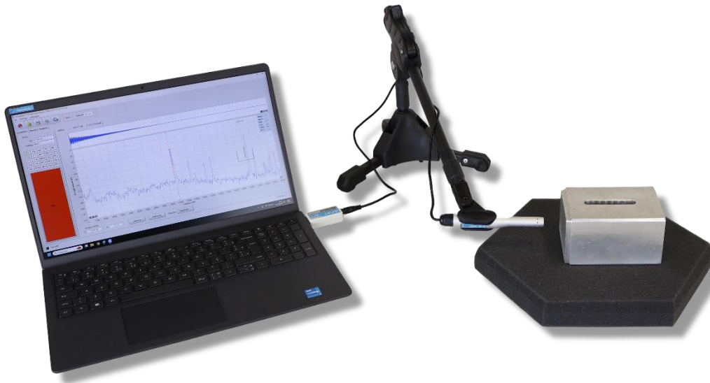
Figure 37 - Arrangement for determining the frequency of a 20 kHz rectangular ultrasonic horn for tuning.
