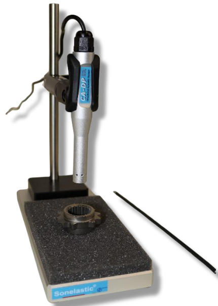
Figure 43 - Arrangement of the Acoustic Sensor CA-DP and SB-AP support for determining the resonance spectrum of a sintered powder metal part.
