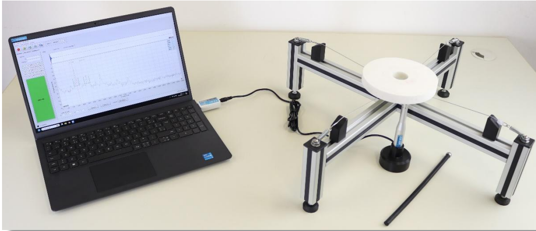
Figure 45 - Arrangement of the CA-DP Acoustic Sensor and SX-PD support for determining the resonance spectrum of a small grinding wheel.
