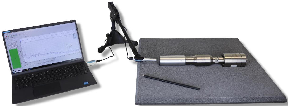
Figure 35 – Arrangement of the Acoustic Sensor CA-DP and medium-sized tripod for basic modal analyses of a 20 kHz ultrasonic welding stack.
