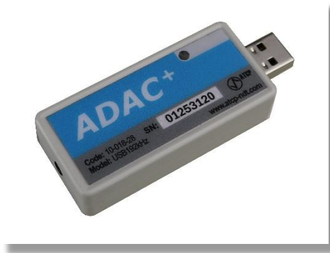
Figure 26 – ADAC+ acquisition device, developed and manufactured by ATPC Physical Engineering. The maximum sampling rate of ADAC+ is 384 kHz.
