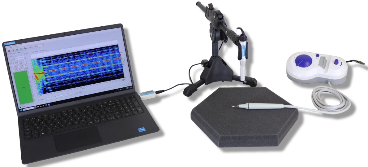
Figure 39 - Arrangement for determining the frequency behavior of an ultrasonic dental scaler during start-up.
