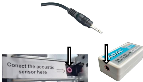
Figure 13 - Acoustic sensor TRS P2 / 3,5 mm plug, audio input from a XONAR acquisition board installed on the rear panel of a DELL computer, and audio input from the ADAC acquisition module.
